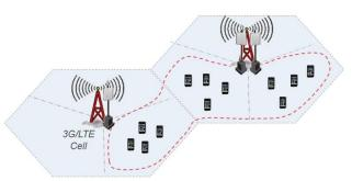
Co-locate A8-Ein with existing 3G/LTE cell site to offload traffic for an almost identical cell area.
