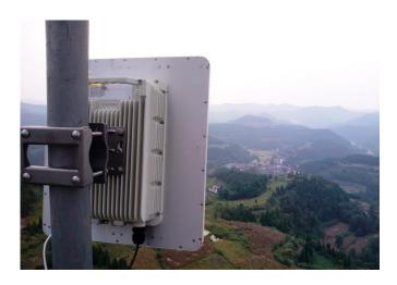
The A8-Ein is a multi-radio base station utilizing 8x8 MIMO smart antenna technologies and a patented signal processing algorithm to provide the industry's best coverage per base station, especially in non-line-of sight (NLOS) environments. The multi-beam antenna array of the A8-Ein is designed to provide up to 5 times the range and 10 times the per site coverage as standard access point. Accordingly, up to 90% fewer installation sites for the same coverage area.
